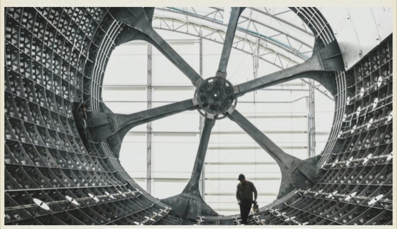
This is the outside of the cylindrical TOOL called "the mandrel." Robots wrap layer upon layer of *carbon-fibre* tape around the mandrel to form a 30-foot-wide "barrel section" of the spaceship.
